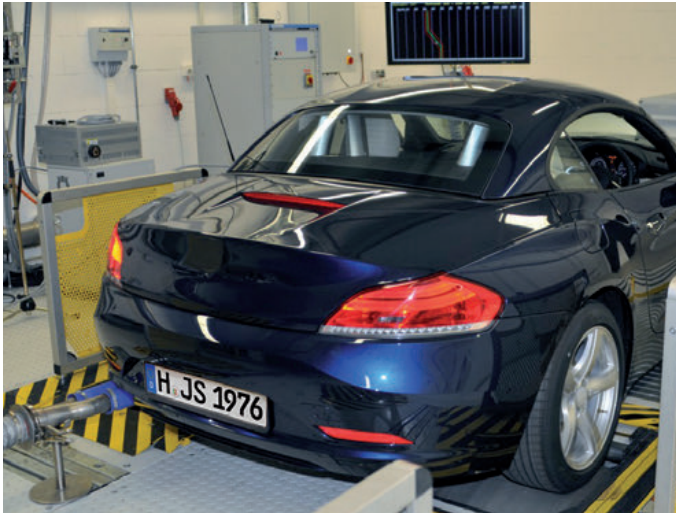
Cross-validation according to ECE guidelines and eco-label requirements on a certified dynamometer.
